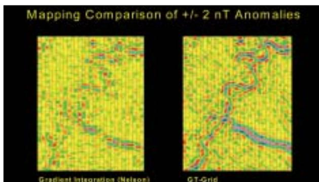
**Figure 9** Comparison of gridding techniques with low amplitude anomalies.
