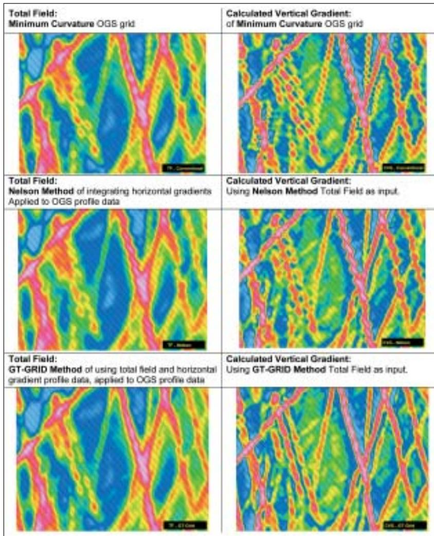
**Figure 8** A demonstration of three gridding techniques using the Ontario Geological Survey (OGS) Kapuskasing-Chapleau aeromagnetic survey data, with measured horizontal gradients. The profile data is identical for each map, only the gridding method is changed. The vertical gradient was calculated in identical fashion from each total field.
